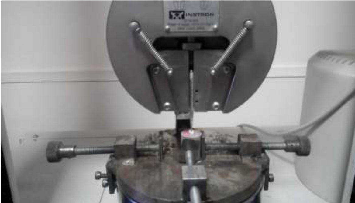
Figure 4: Tooth being tested for vertical fracture resistance
