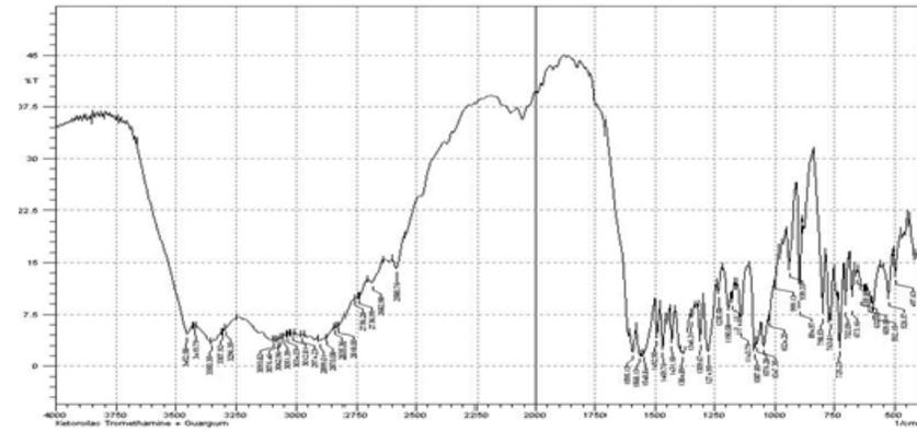
Figure 2: FT-IR spectra of Ketorolac tromethamine and Guar gum
