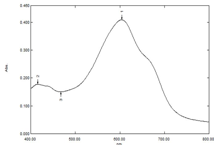
Figure 3: Absorption spectra of Deferasirox with MBTH reagent.  $\lambda_{\text{max}}$  at 603 nm
