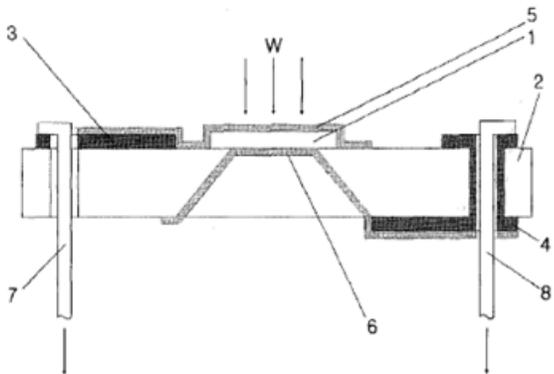
Figure 2: 1-pyroelectric plate; 2-dielectric substrate, 3,4-metal layers, 5,6-electrodes, 7,8- output leads.
