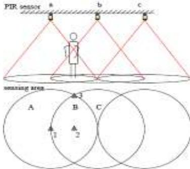
Figure 1: Resident-detection method using PIR sensors.
