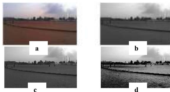
Figure 2: (a) Original Frame (b) Gray scale image (c) Gabor Filter Output (d) Histogram Equalization
