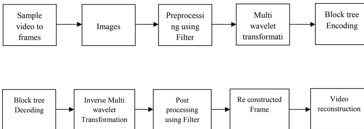
Figure 1: Video compression System Block Diagram
