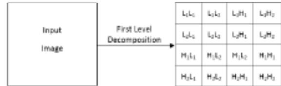
Figure 5: Representation of Multi Wavelet Decomposition of Input Image
