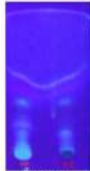
Fig. 4.1 a T.L.C. observed under UV 366 nm
