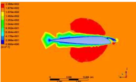
Figure 11: Velocity distributions at 1° control deflection
