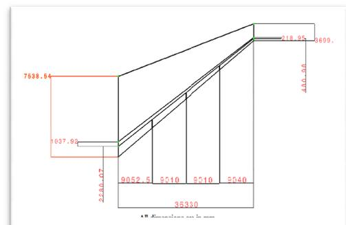
Figure 7: Dimensions of the wing model
