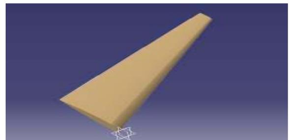
Figure 6: Wing without control surface
