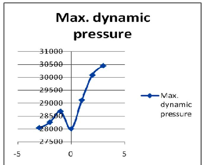
Figure 13: AOA Vs maximum Dynamic pressure
