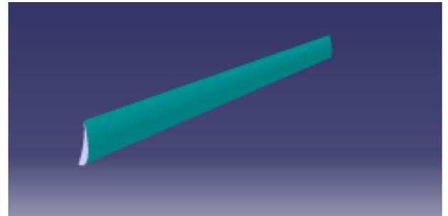
Figure 4: 3<sup>rd</sup> Leading edge control surface
