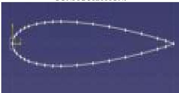
Figure 1: NACA 0012 Airfoil
