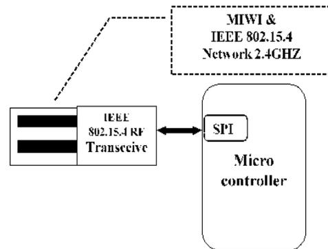
Figure 3: Block Diagram of Reference motes
