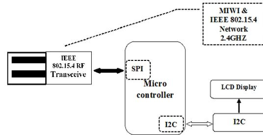
Figure 2: Block Diagram of Display Mote
